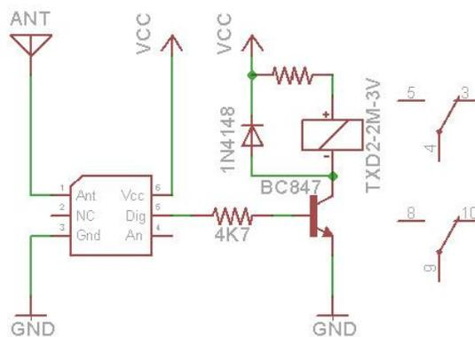
**NOTES** : - BC847 transistor can be replaced by any suitable transistor.
